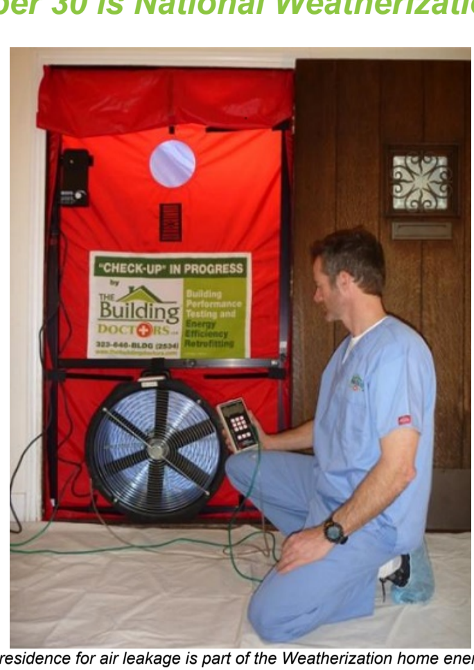
Testing the residence for air leakage is part of the Weatherization home energy audit.
